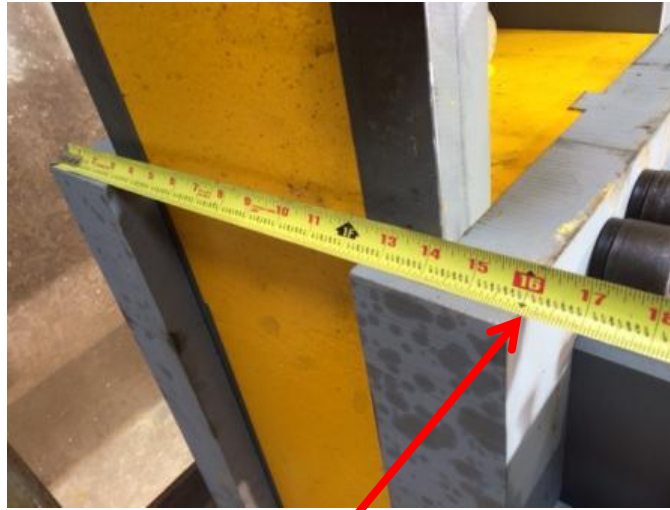
Measurement of the overall distance between the Grabber Torque Box Top (M800167) and Grabber Torque Box Bottom (M800128).
